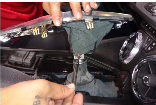
8. Align the screw holes on shifter handle and the stick. Start both flat head screws (2), then tighten them.
