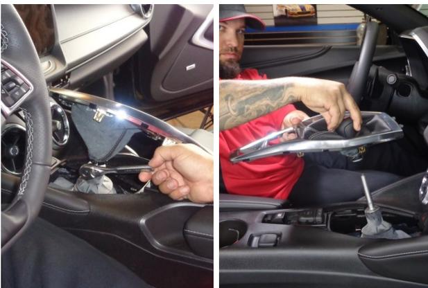
2. Remove the screw from the base of shifter handle, then lift the handle, boot and bezel off the stick.
