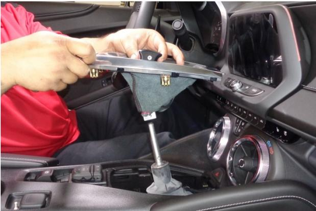
7. Install the handle body onto the shifter stick.
