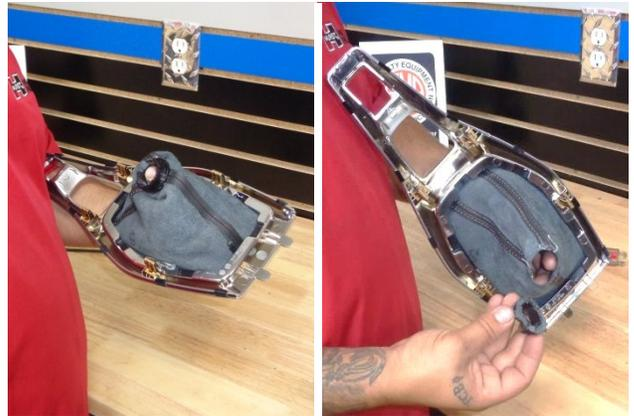
4. The plastic collar is glued to the shifter boot. Carefully separate the collar from the boot.
