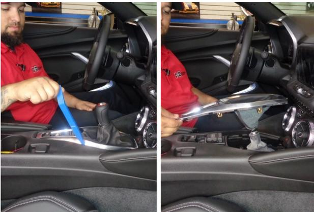
1. Use a plastic trim tool to separate the shifter bezel from the console, then lift the bezel straight up.
