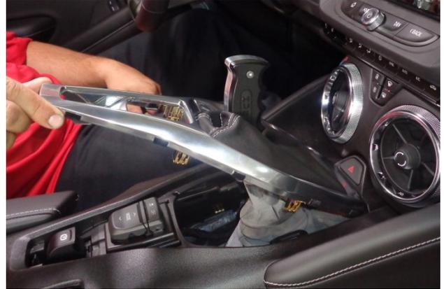
9. Reinstall the shifter bezel in the console.
