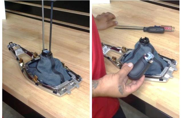
3. Use 2 flat-tip screwdrivers to separate the shift handle from the plastic collar.
