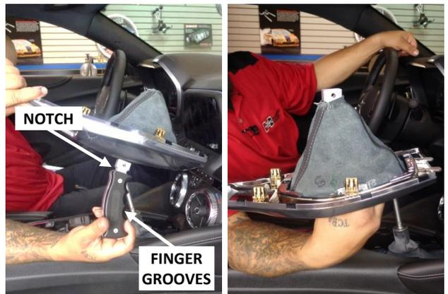
5. With the finger grooves pointing forward, work the base of the shift handle (1) through the opening in the shifter boot until the opening surrounds the notch at the base of the shift handle.
