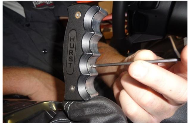
10. Install and tighten the set screw (3) in the front of the shifter handle.
