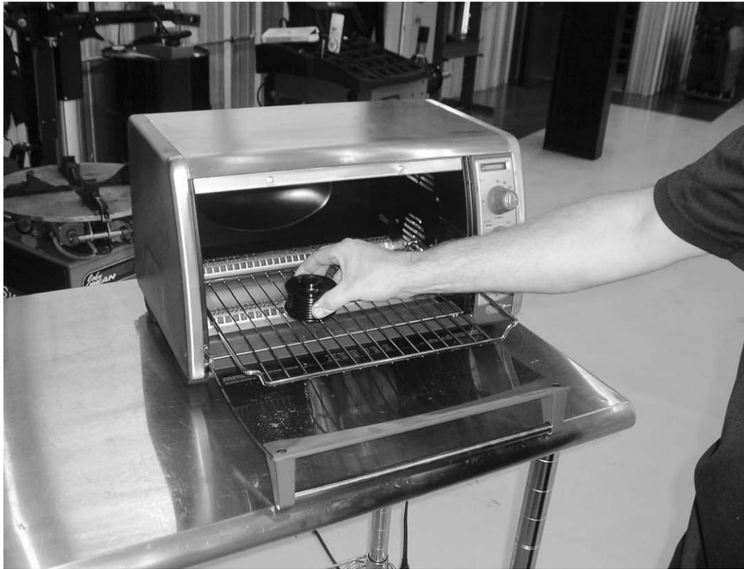
1) Place APR pulley in 350° toaster oven (or equivalent) for one hour (or more). Place the oven on a cart to ensure it can be moved close to the vehicle. Exceeding 350° can damage the finish on the pulley.
