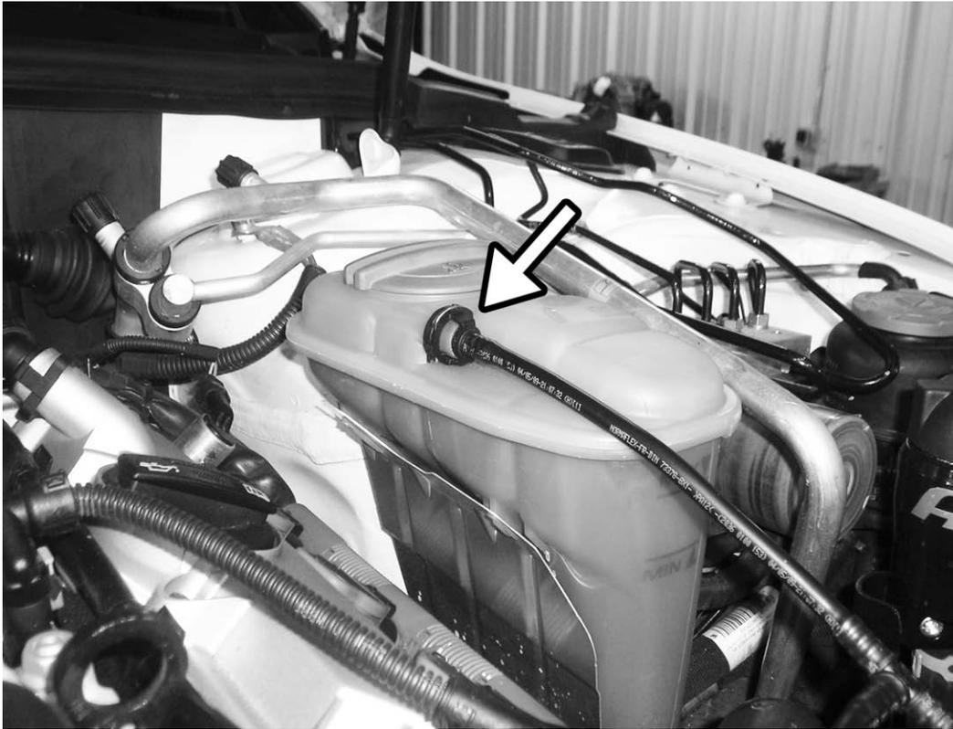
33) Reconnect coolant bleed line to expansion tank.
