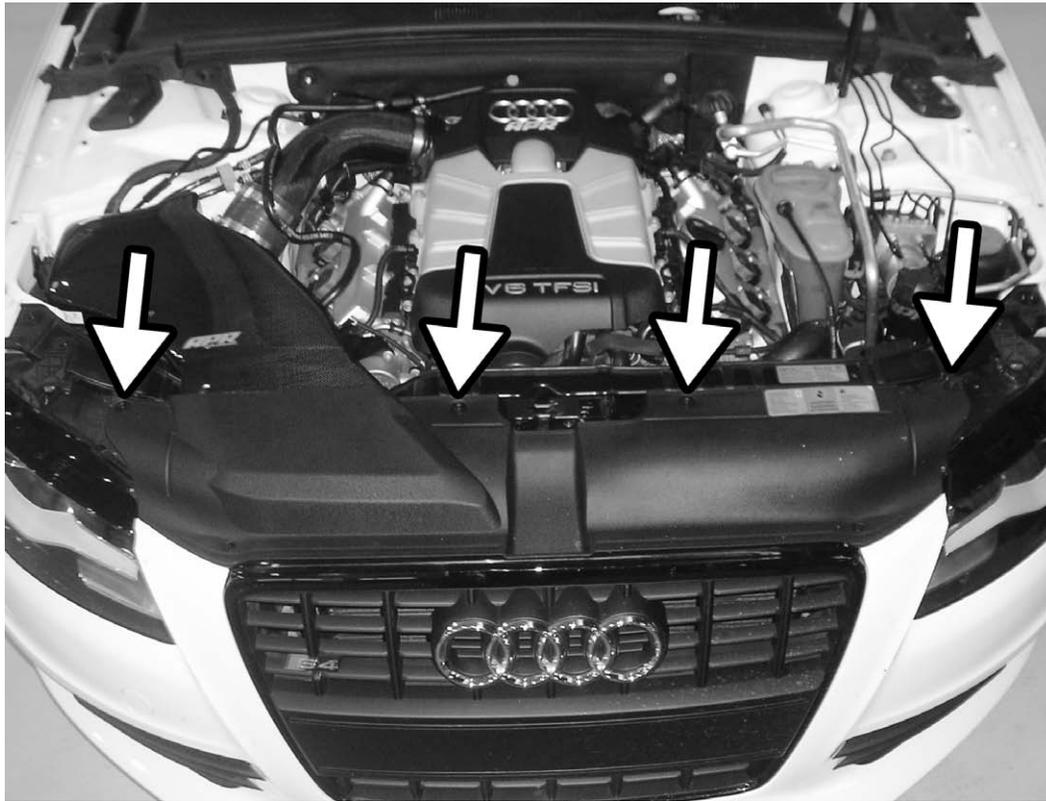
7) Remove 4 T30 Torx screws from upper bumper trim cover and remove the cover.
