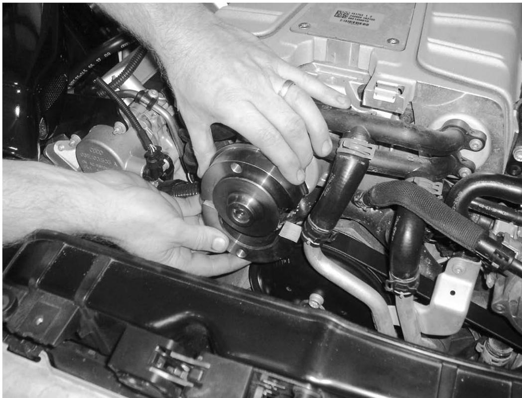
21) Install the supplied “half-moon” pieces around stock pulley. One half moon set fits the stock pulley and the other set fits the APR pulley.
