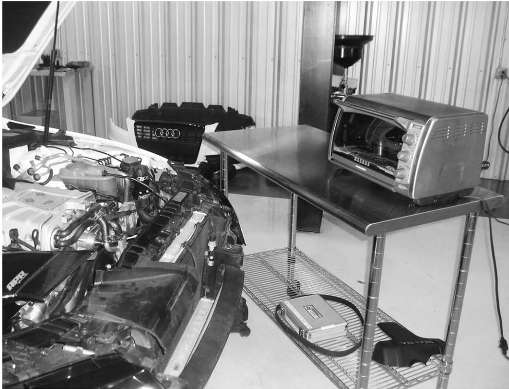
27) Now that the stock pulley is removed, move the oven close to car so that pulley can be installed as quickly as possible.
