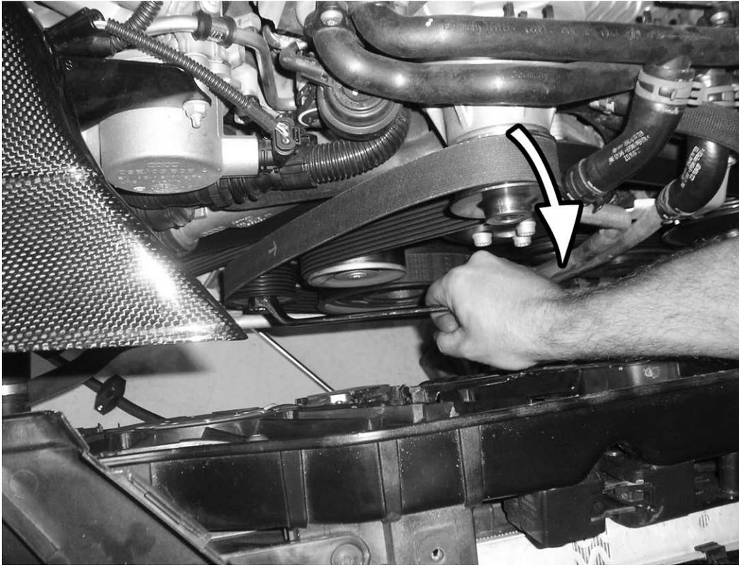
19) Using a 16mm wrench, release tension on supercharger's belt tensioner by pushing down and carefully remove the belt.
