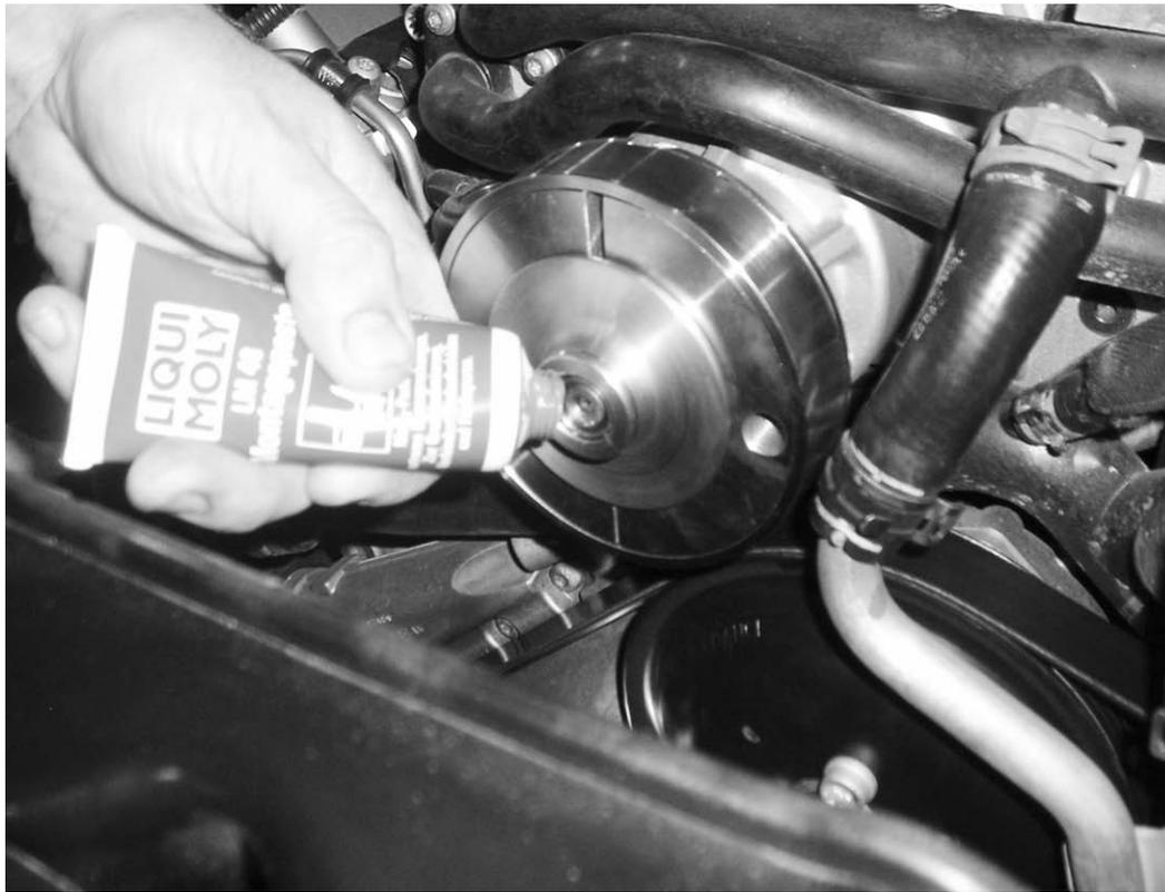
23) Generously apply supplied Liqui Moly to end of the supercharger's drive shaft.
