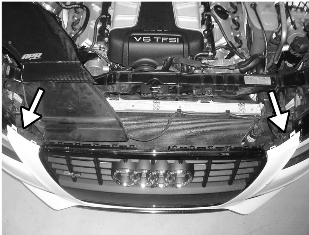
39) Reinstall 2 T25 Torx screws from top of bumper cover.
