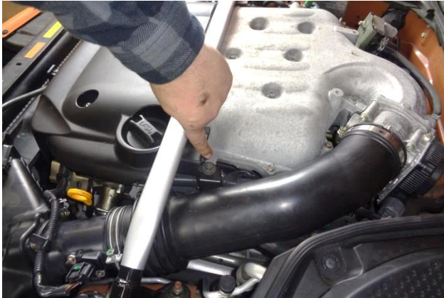
7. Remove the air duct bracket bolt.
