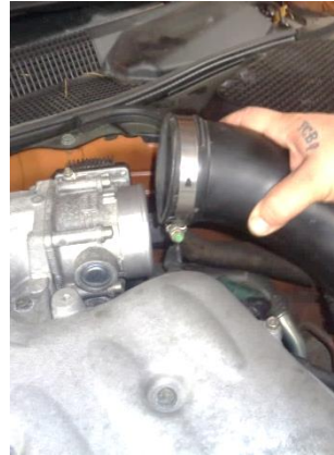
10. Separate the duct from the throttle body and the airbox, then carefully roll the duct slightly away from the engine.
