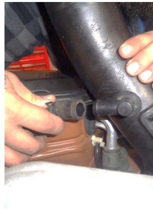
11. Loosen the pinch clamp, separate the PCV line from the intake duct and remove the duct from the vehicle. Retain the pinch clamp for use at Step 27 .
