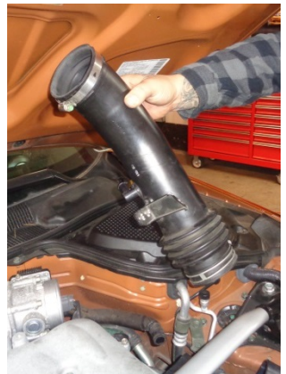
11. Loosen the pinch clamp, separate the PCV line from the intake duct and remove the duct from the vehicle. Retain the pinch clamp for use at Step 27 .
