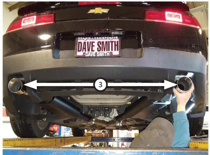
9. Adjust exhaust components for fit; maintaining ½" clearance and compensating for suspension, travel and vibration, then tighten all clamps. Finally, fit (x6) **hanger keepers (5)** onto each sideways hanger.
