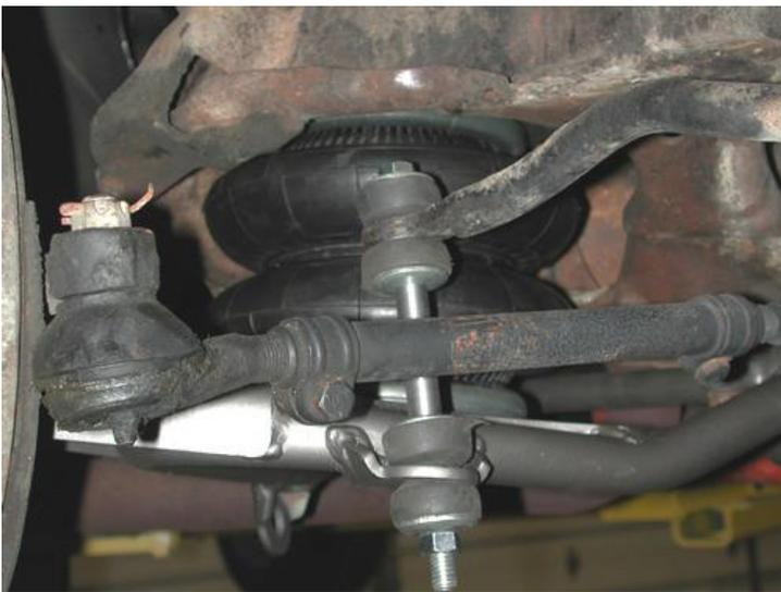
6. The sway bar end link must be shortened to 2" tall optimize clearance and alignment. Use the shorter 3/8" x 6 1/2" bolt supplied. (Discard if using RideTech MuscleBar)
