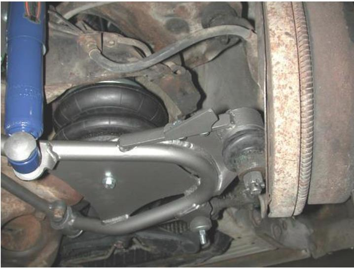
3. Bolt the lower StrongArm shaft to the frame. 7/16" x 2" bolts, lock washers and flat washer will be used to fasten the aluminum clamp to the frame.
