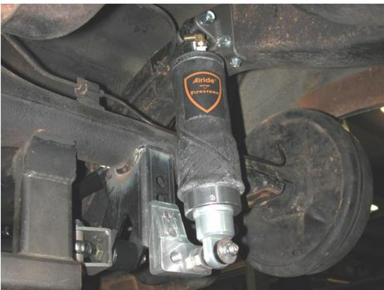
22. Apply thread sealant onto the air fitting and screw it into the top of the shockwave. Air fitting location can be moved by rotating the bellows assembly separate from the shock.
