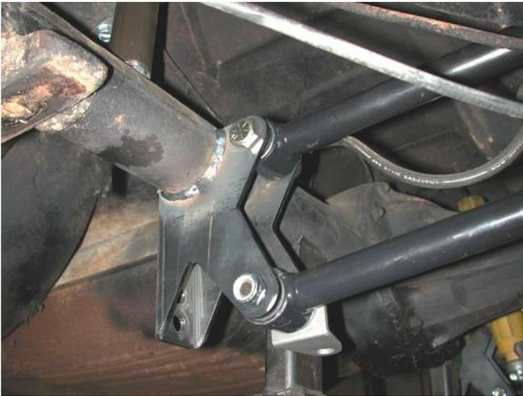
13. Insert the R-Joint spacers into the R-joint with the small OD inserted into the R-Joint center pivot. Install the 4 link bars into the crossmember and axle bracket. Use the 5/8" x 2 3/4" bolts and nyloks supplied.
