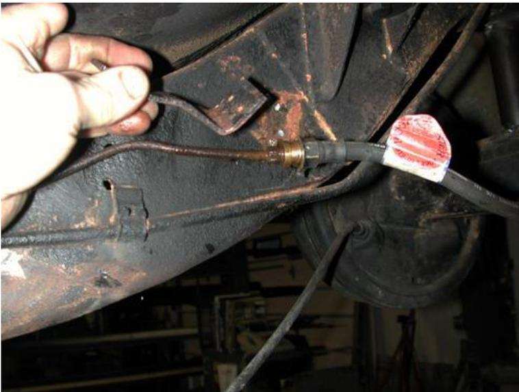
4. The rear brake line bracket on the passenger side frame rail must also be removed.
