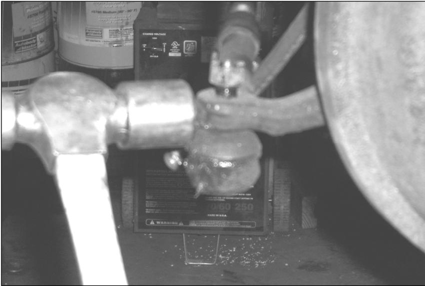
If you remove the calipers but leave the hoses attached, supporting them to avoid stressing the hoses, you won't even need to rebleed the brakes!
