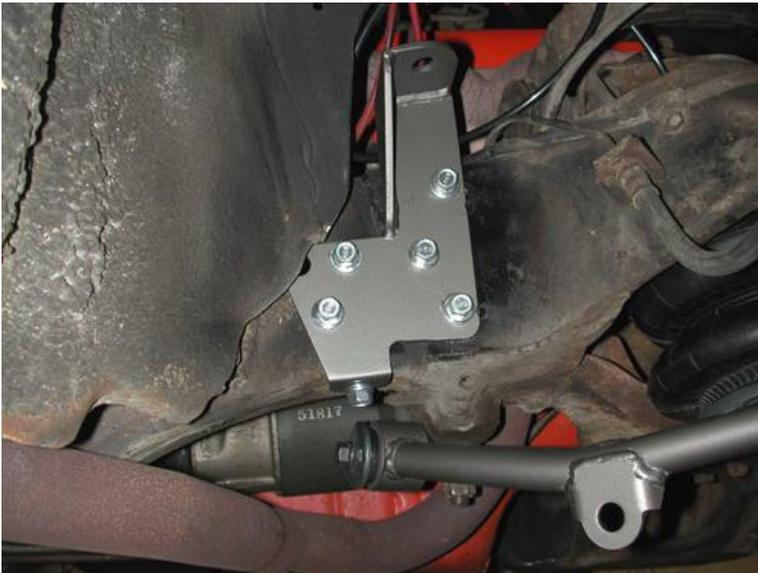
1. Position the upper shock mount on the frame so the hole in the bracket aligns with the hole in the side of the frame and the tab is against the bottom of the frame. You may have to trim some of the inner fender well for clearance. On manual shift cars you may have to trim the bottom of the Z-bar clutch bracket on the driver's side.
