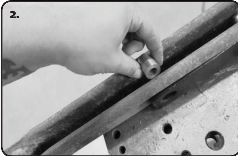
**2.** Insert the Supplied Spacer into the inside of the Control Arm at the Hole Locations. These Spacers will get Clamped in place by the Mounting Hardware after the SwayBar is installed. These can be welded in place if desired.
