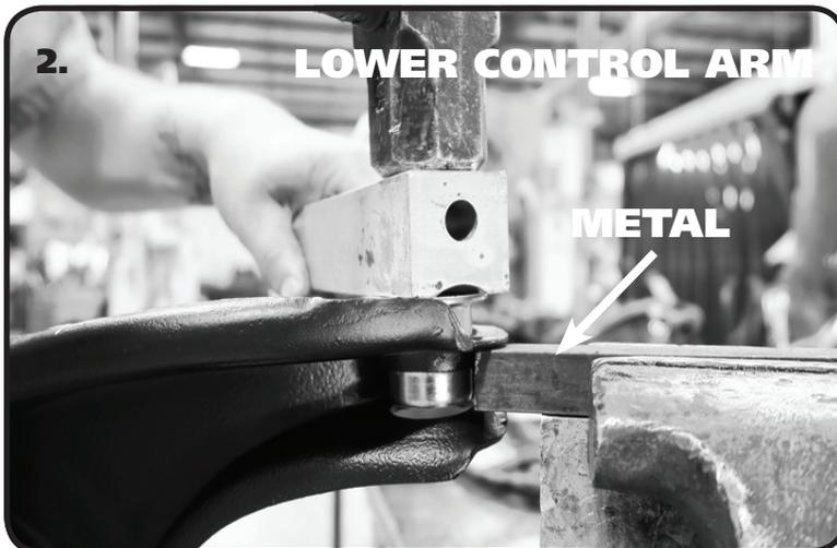
**3.** Use another Piece of Metal or Strong Wood to Drive the Outer Shell into the Control Arm until the Shell stops against the Control Arm.
