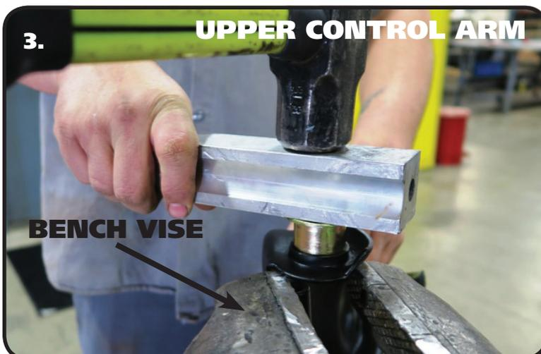
**The Upper Control Arm requires spacers to be ran on the attaching bolts. The kit includes a 1/4" Aluminum Spacer for each front bolt and a 3/4" Aluminum Spacer for each rear bolt. It is necessary to run these spacers.**
