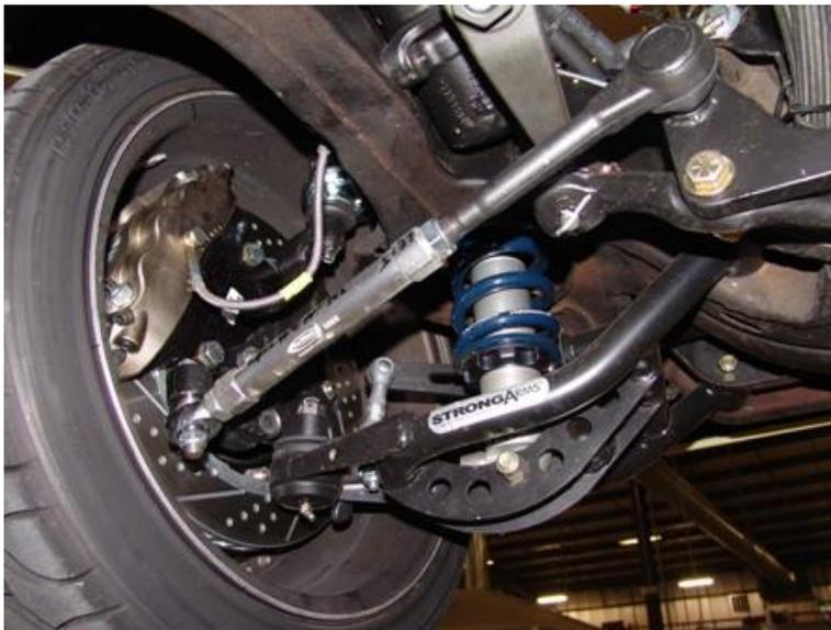
4. Check clearance between the upper spring retainer and stud base with the factory coil spring retainer this area may need trimmed to get full shock movement.
