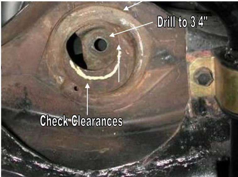
1. Inspect the factory welds attaching the upper shock bracket to the frame. Re-weld if necessary.
