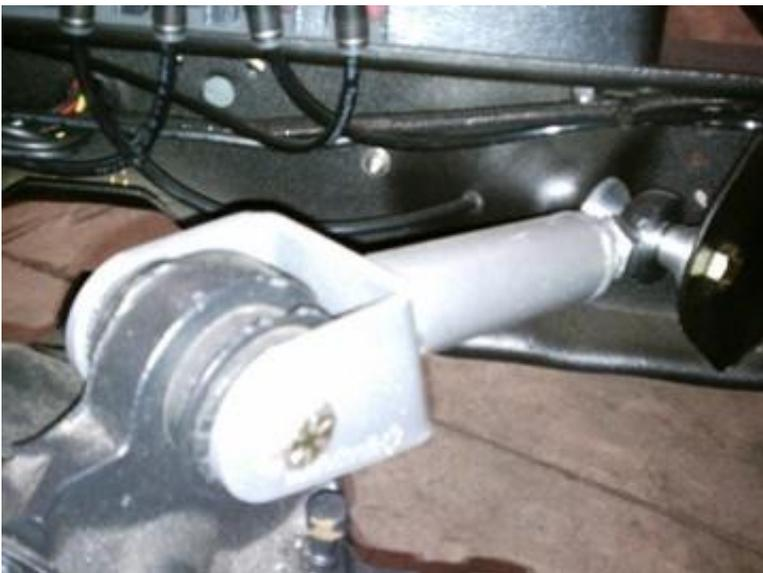
4. Fasten the other end of the bar to the axle using a 1/2" x 3 1/2" bolt and Nylok nut.
