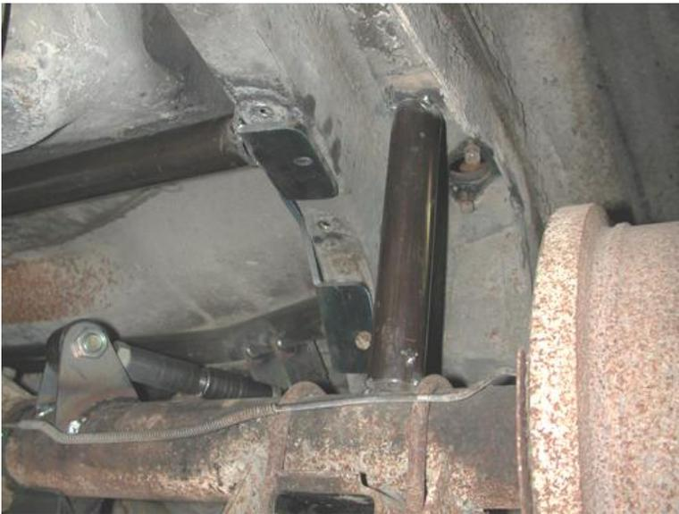
**14.** One helpful trick to help maintain ride height and pinion angle while adjusting is to tack weld a spacer between the axle and the outside of the frame as shown in the picture. This spacer should be 8 3/8" tall giving the Shockwave an eye-to-eye measurement of 14 1/2" to 15".
