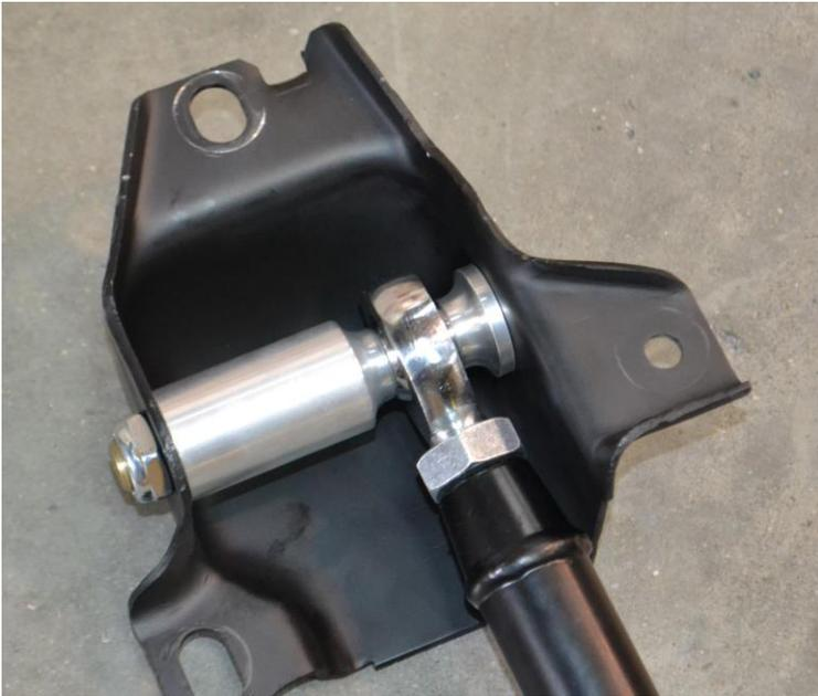
6. The heim end bar setup is designed to be offset to the inside of the car. The bolt hole in the mounting bracket has to be drilled out to 5/8" and the new longer bolt is used. The wider spacer is used on the outside with a narrow spacer on the inside. The bar is offset to provide better wheel and tire clearance.
