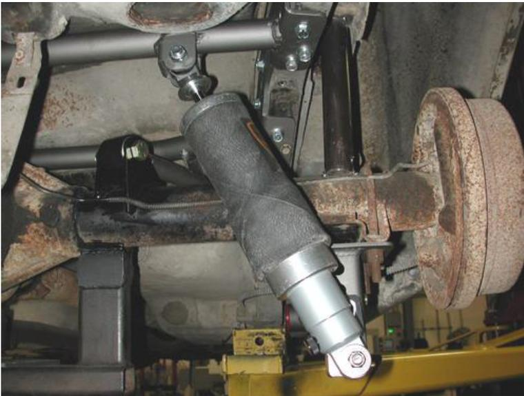
**18.** Apply thread sealant to the air fitting and screw it into the Shockwave.
