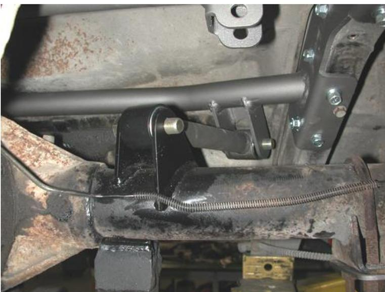
11. Check the length of the upper bar; it should be 9 1/4" C-C. Bolt the axle tabs to the setting jig (**The setting jig is explained on the next page**) . (Longer ears to the front) Then place the other end of the jig into the cradle. Both ends use a 5/8" x 2 3/4" and should not be fully tightened yet. For now just the let axle tabs sit on the axle.
