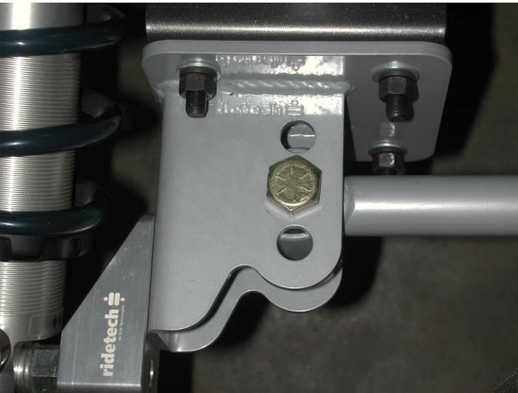
8. The lower axle bracket will be fastened to the leaf spring pad using the factory U-bolts. It is offset to the inside of the car. New 7/16" nylocs are supplied.
