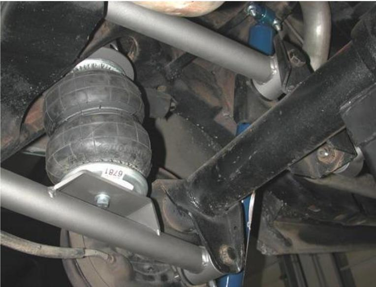
1. Replace the factory upper trailing arm with the StrongArms. 5/8" x 3 3/4" bolts and Nylok jam nuts are supplied to replace the factory hardware. A 5/8" ID x 1.031" long spacer will need to be inserted into each side of the R-Joint.
