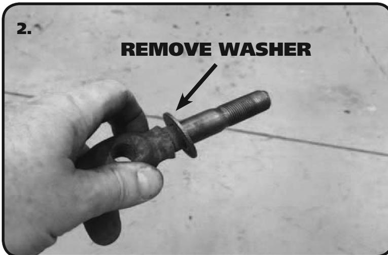
**2. UPPER CONTROL ARM:** The Upper Control arm has an inner washer on the cross shaft that needs to be removed before installing the Delrin Bushings. Remove each of the 4 washers from the cross shaft.
