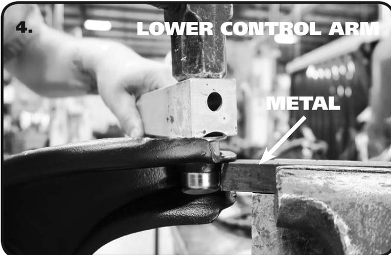
4. Disassemble the Bushing being installed. If installing Bushings in the Upper Control Arm, insert the Cross Shaft before installing any Bushings. Support the Back Side of the Flange the Bushing is being Installed in. Use a STIFF piece of Metal clamped in a Bench Vise for the Lower Control Arms (Image 4). The Upper Control Arm can be supported by either the same piece of Metal or by the Bench Vise with the Jaws opened wide enough to let the Bushing Shell pass through (Image 5).
