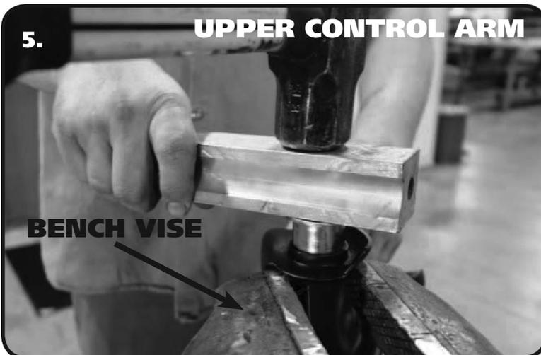
5. Use another Piece of Metal or Strong Wood to Drive the Outer Shell into the Control Arm until the Shell stops against the Control Arm.
