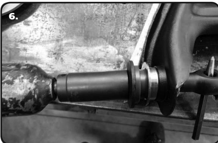
6. Press the Inner Sleeve into the Delrin Bushing and little tap them into the Shells. TAP THE CENTER OD THE BUSHING/SLEEVE, DO NOT HIT THE OUTER FLANGE.
