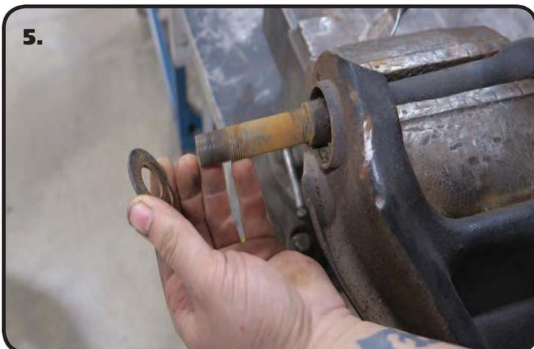
**5. UPPER CONTROL ARM:** The Upper Control arm has an inner washer on the cross shaft that needs to be removed before installing the Delrin Bushings.
