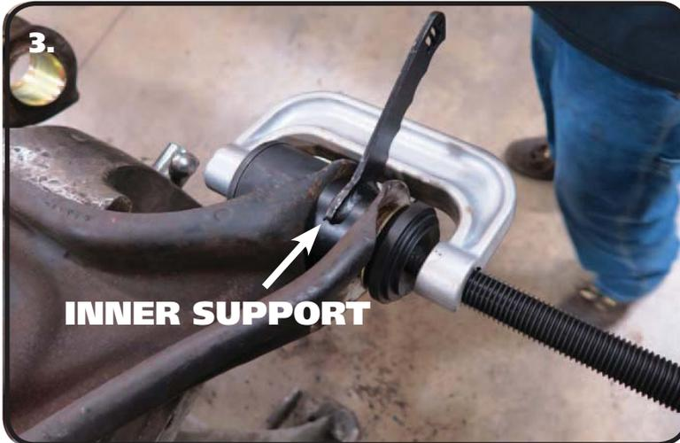
**3. LOWER CONTROL ARM:** The Lower Control Arm's Outer Shells can be installed before the Cross Shaft is installed, it will slide through the Shells. We used a C-clamp style tool to install our bushings. Most auto parts stores have these as a loan-a-tool. When pressing the Outer Shell into the arm, **be sure to support the inside of the arm to keep it from crushing.** Press the shell in until it bottoms against the control arm.
