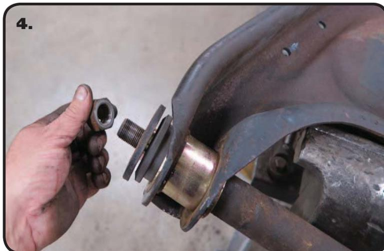
**4.** Insert the cross shaft into the control arm by sliding it through the Outer Shells installed in the arms. Push the Inner Sleeve into the Delrin Bushing. Push the Delrin Bushing/Inner Sleeve assembly into the Outer Shells. They will go in partially. Install the OEM washer and nut on each end of the cross shaft. Tighten the Hardware on each end until the Delrin Bushings are bottomed out against the lip of the Outer Shell installed in the control arm.
