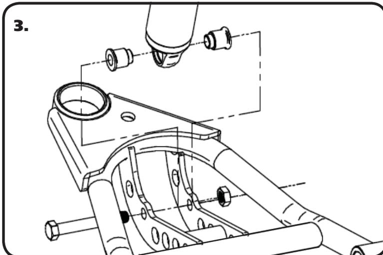
**Install the ShockWaves/CoilOvers at this time. Refer to the CoilOver instructions for Assembly.**
