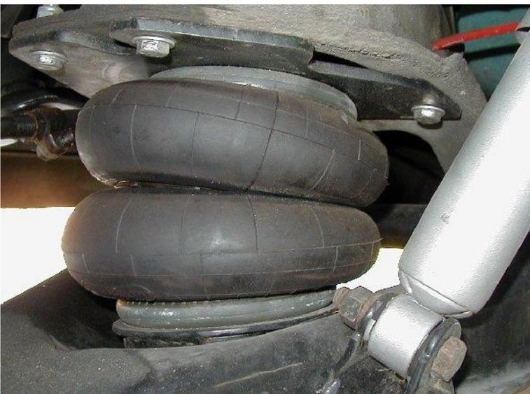
5. Bolt the lower bracket to the air spring using two 3/8" x 3/4" bolt, lock washer and flat washer.
