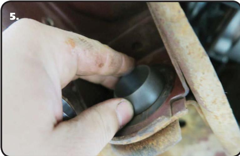
7. Refer to **(Figure 6)** for the Delrin Strut Rod Bushing assembly order. The Delrin Strut Rod Bushing will insert into the frame bushing hole with the rounded side of the bushing outward. A Bushing needs to be installed on both the front and rear side of the frame. With a Delrin Strut Rod Bushing on each side of the frame, insert the INNER Sleeve in the Bushings. This will help hold them in place.
