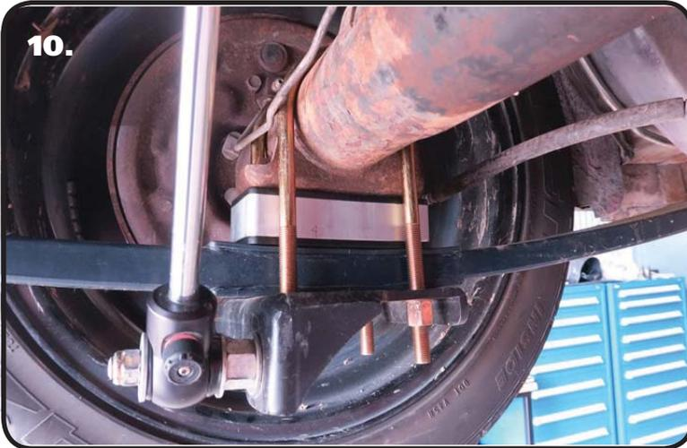
10. Tighten the Bushing hardware, torquing it to 75 ftlbs. The Delrin Bushings will not bind, so it isn't necessary to have the car at ride height.
