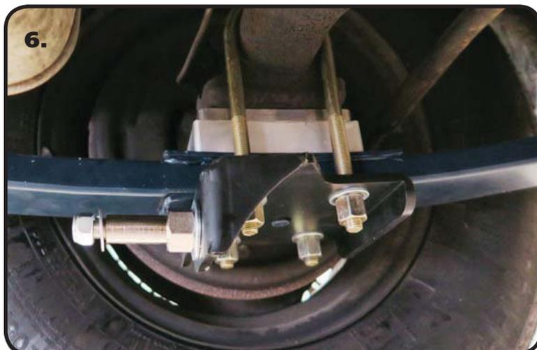
**6.** The Lower Shock is Bolted to the Lower Shock Mount using the supplied Shock Stud. Install the Studs into the Lower Mounts with a Washer on each side of the Mount. Slide a Washer onto the Stud. Jack the Rear Differential up until the Shocks can be slid onto the Shock Stud. Slide the Shock onto the Stud with the Adjuster Knob pointing inward. Install the supplied 7/16" Flat Washer and Nylok Nut onto the Threads and tighten.
