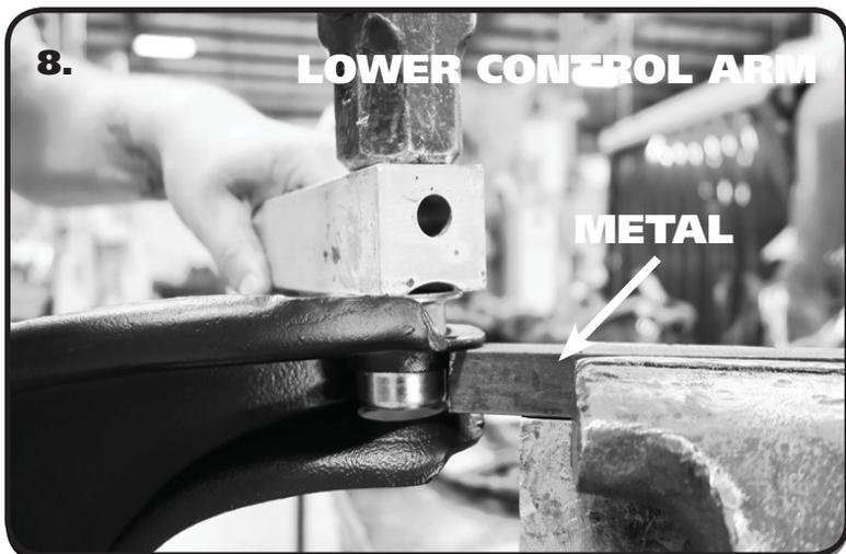
8. Remove the OEM Lower Control Arm Bushings. This Kit contains 2 different sizes of Lower Control Arm Bushings. Use your control arm to determine which size is needed. Use (Image 9) to help with determine the Bushing assembly order. Support the back side of the Flange the Bushing is being Installed in. Use a piece of metal clamped in a Bench Vise for the Lower Control Arms.
