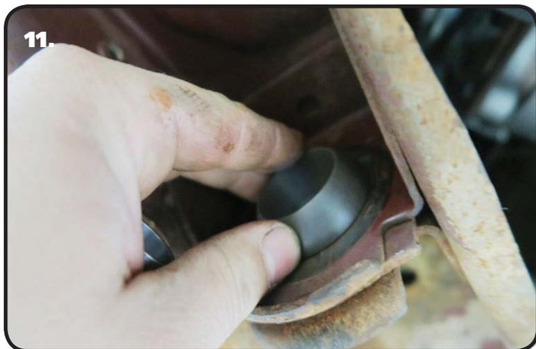
11. Refer to **(Image 13)** for the Delrin Strut Rod Bushing assembly order. The Delrin Strut Rod Bushing will insert into the frame bushing hole with the rounded side of the bushing outward. A Bushing needs to be installed on both the front and rear side of the frame.
