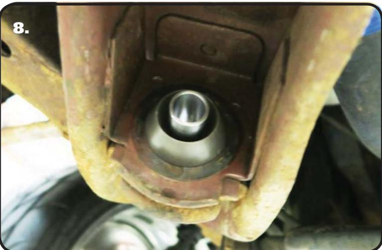
**8.** Install the Inner Sleeve in the Strut Rod Bushings. Center the Sleeve in the Bushings, this will also help hold the Bushings in place during reassembly of the strut rod.
