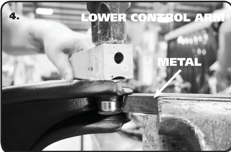
4. Remove the OEM Lower Control Arm Bushings. This Kit contains 2 different sizes of Lower Control Arm Bushings. Use your control arm to determine which size is needed. Use **(Figure 9)** to help with determine the Bushing assembly order. Support the back side of the Flange the Bushing is being Installed in. Use a piece of metal clamped in a Bench Vise for the Lower Control Arms.
