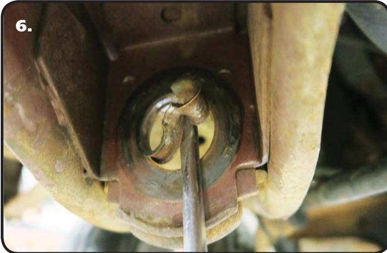
**6.** A Delrin Bushing setup for the strut rod is also included in this kit. The liner that is installed in the frame hole has to be removed. Use a chisel to distort it and remove it. In **(Figure 10)** we distorted it from the bottom edge and removed it.
