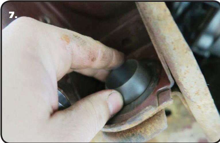
**7.** Refer to **(Figure 13)** for the Delrin Strut Rod Bushing assembly order. The Delrin Strut Rod Bushing will insert into the frame bushing hole with the rounded side of the bushing outward. A Bushing needs to be installed on both the front and rear side of the frame.
