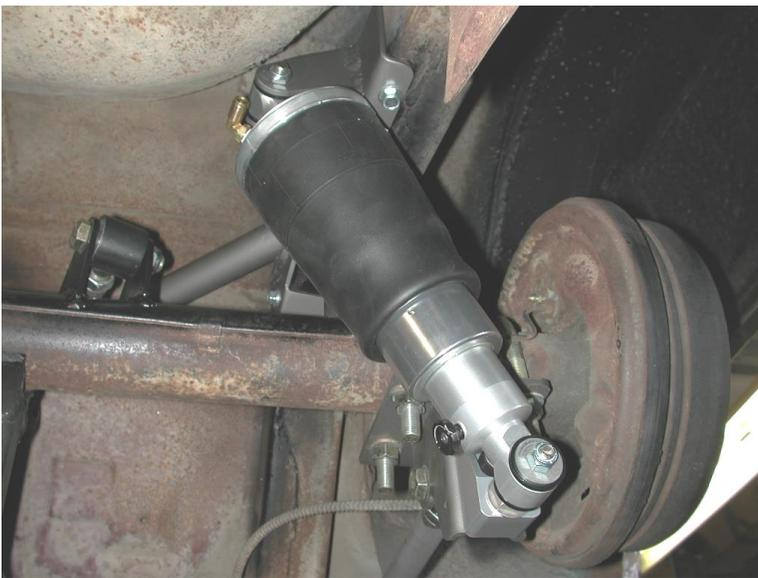
16. This must all be set at **ride height**, which will occur with 14.5" from c-c on the Shockwave mounts. As you can see in the above picture, we have tack welded a 5" long spacer between the axle and frame to maintain ride height, axle center, and pinion angle while welding in the tabs.
