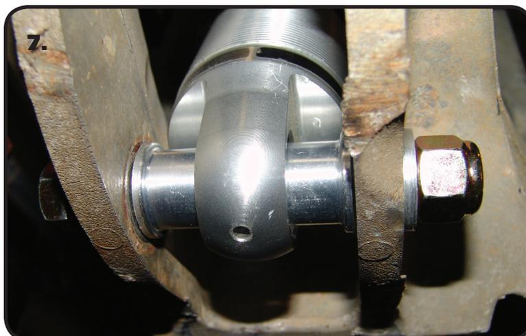
7. With the **WIDE** spacers installed in the lower ShockWave Bearing, insert the ShockWave into the Lower Control Arm. Align the hole in the ShockWave with the hole in the T-bushing. Insert the 1/2" x 3 3/4" Hex Bolt into the mounting hole in Lower Control Arm. Install a 1/2" Nylok Nut onto the Bolt and tighten.
