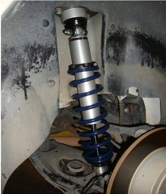
8. Attach the eyelet to the lower control arm using a wide spacer in each side of the bearing. Attach the eyelet using the OEM bolt and OEM nut.
