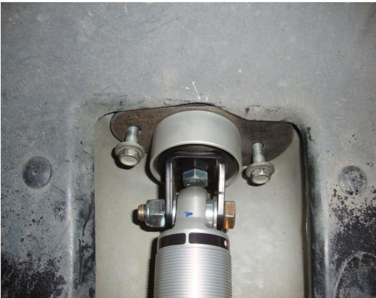
6. Install the CoilOver assembly into the upper mount with a narrow spacer in each side of the bearing. Attach it to the upper mount using a  $\frac{1}{2}$ " x  $2\frac{1}{2}$ " bolt.
