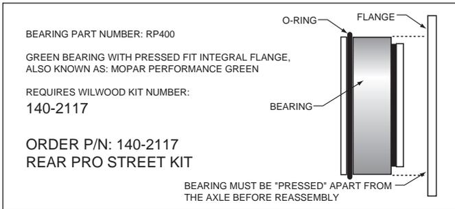
**Figure 1. Press Fit Flange Bearing Configuration**
