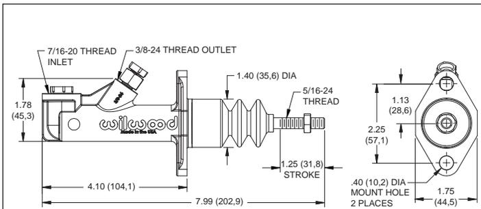
Figure 1. GS Compact Remote Master Cylinder, Physical Characteristics
