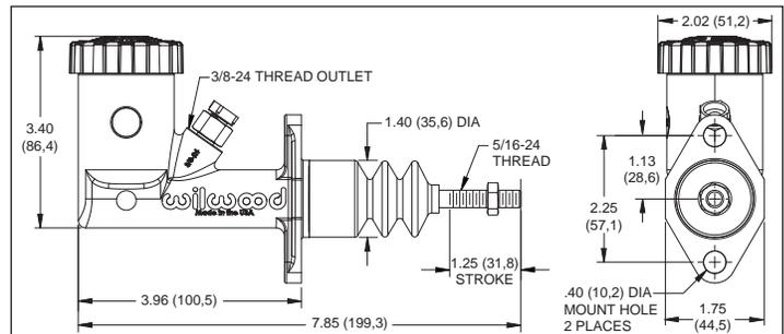
Figure 2. GS Compact Integral Master Cylinder, Physical Characteristics
