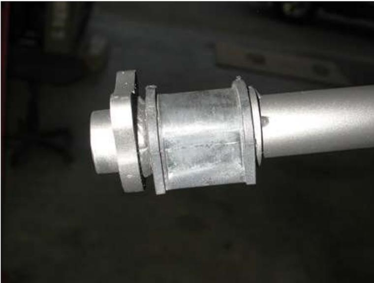
4. Apply lithium grease to the poly bushing then slide it over the sway bar.
