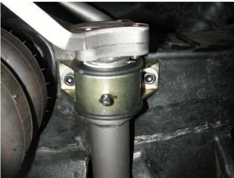
5. Secure the sway bar to the frame with two 5/16" x 1" Socket Head Cap Screws, flat washers and Nylok nuts.
