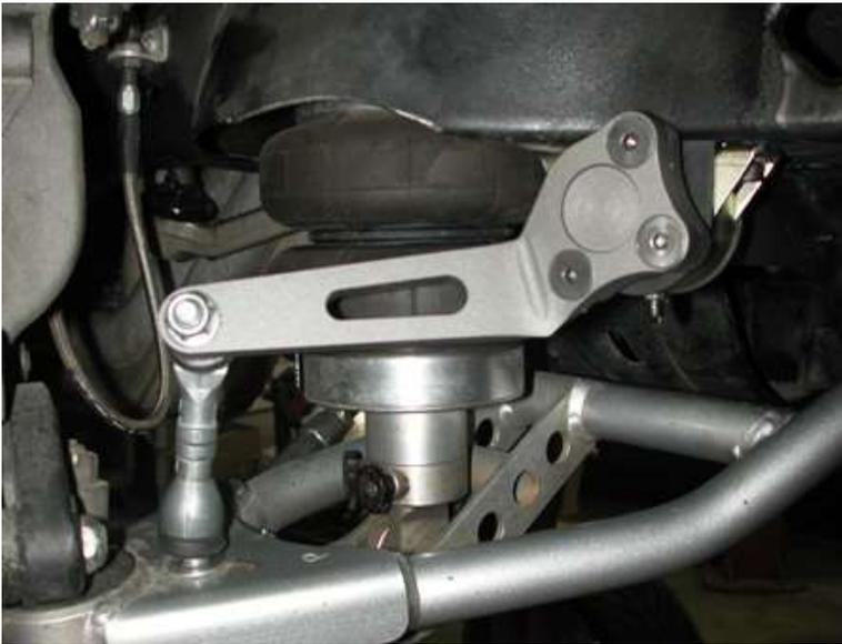
7. Attach the arm to the bar using three 3/8" x 1" Flat Head Cap Screws. **Blue or Green Loc-tite must be applied to the threads of these bolts.**
