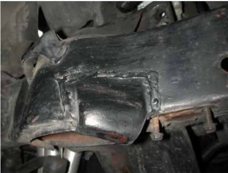
3. On some cars, the compression stop bracket that is welded to the frame will need to be removed to allow clearance for the sway bar arm.
