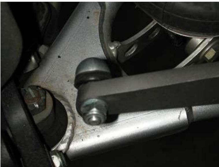
9. Attach the other end of the PosiLink to the sway bar arm with a 3/8" flat washer and a 10mm Nylok nut.
