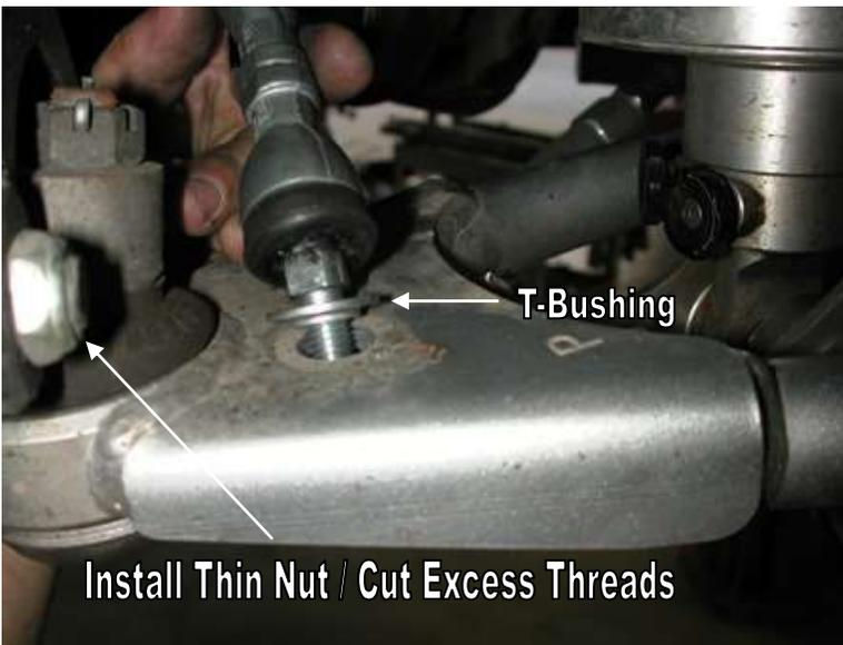
8. The straight end of the PosiLink will attach to the lower control arm. **A "T"-Bushing must be installed on each side of the control arm.** Secure the assembly with a 10mm Nylok nut.
