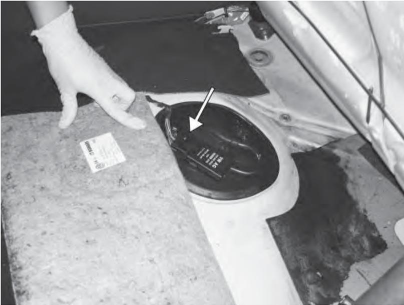
57) Flip up the bottom of the rear seat, but do not remove it. Under a carpet flap, you will see the access to the fuel pump. Disconnect the electrical connector on the plastic cover, and then pry the cover off carefully.
