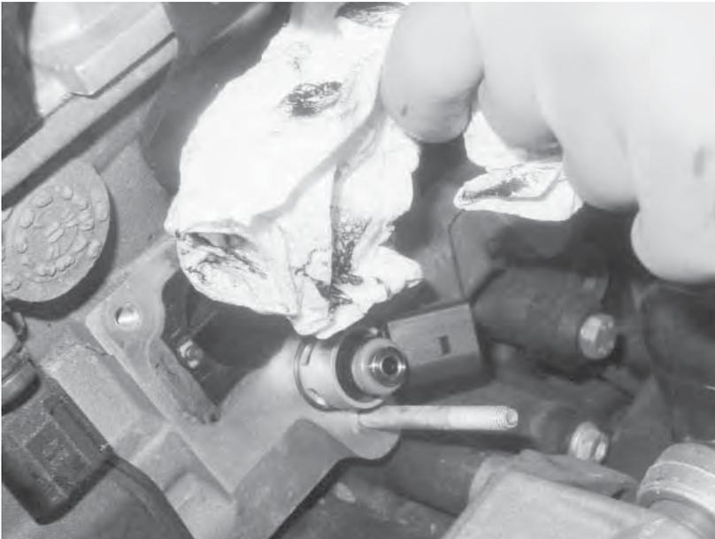
38) Remove the paper or cloth from the intake ports on the block, being careful not to pull the flow separators out of the block.
