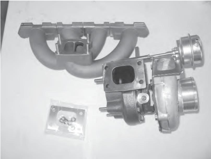
86) On a clean workbench, lay out the APR exhaust manifold, turbocharger, and turbo to manifold gasket set. Make sure all parts are clean and any debris is removed.
