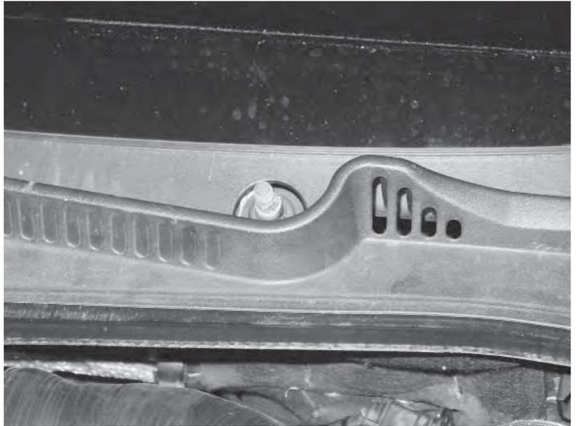
8) Remove the two 10mm bolts from the upper cowl panel. Once removed, unclip the wiring harness that is connected to the backside of the panel. Carefully lift the panel out of the car.
