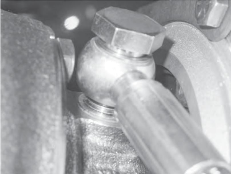
93) Install the other braided steel coolant line on the other side of the turbocharger. Again, install a crush washer on both sides of the banjo fitting, and tighten the 19mm banjo bolt.
