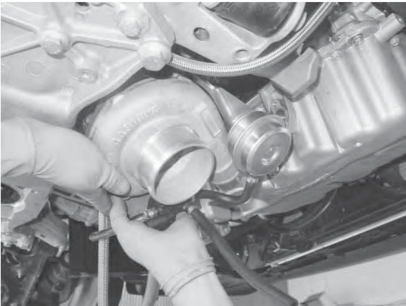
102) Lift the APR manifold/turbo assembly behind the engine as shown. Lift with the downturn end first as high as possible behind the engine, and then rotate the assembly into its correct orientation. Rest the manifold on the lower stock exhaust manifold brackets.
