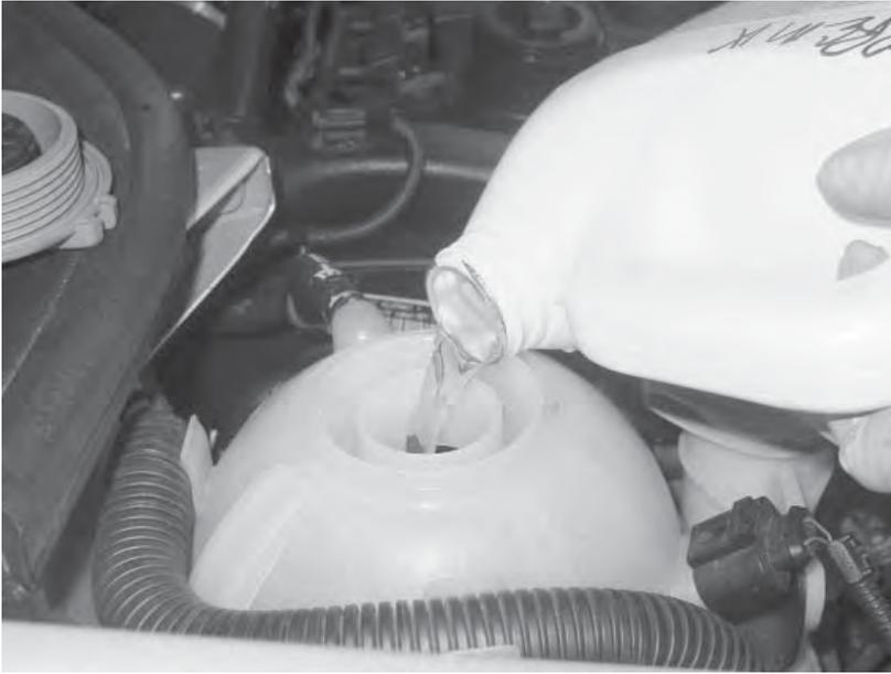
141) Check the engine coolant level and fill if necessary. Reinstall the reservoir cap before the thermostat on the car opens.
