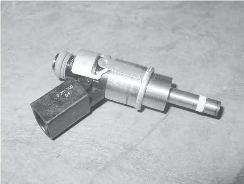
33) Preassemble the APR injectors with the new, supplied injector clips. The gaskets included in the installation kit are not needed with the new APR injectors.
