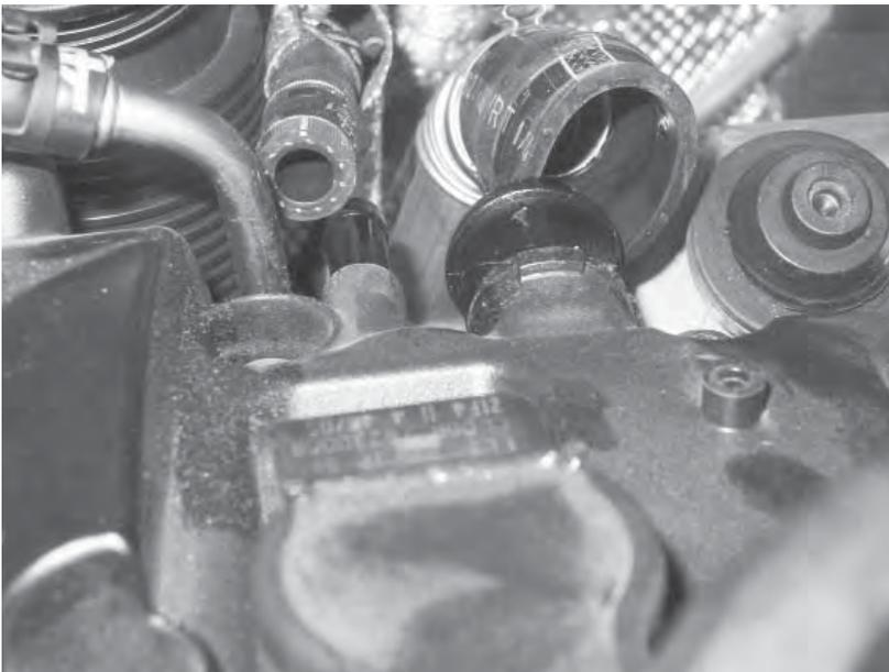
78) Remove the two rubber lines from the back side of the valve cover.
