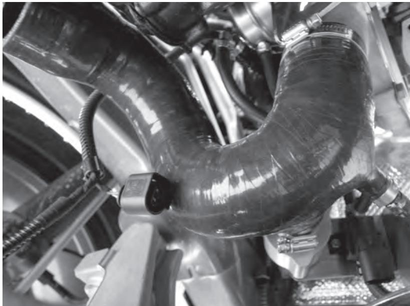
66) Install the compressor outlet hose to the turbocharger with the supplied clamp, but do not tighten the clamp. After sliding the supplied hose clamp on the port of the compressor outlet hose, install the inlet (bottom) side of the diverter valve adaptor into the port. Connect the final vacuum hose from the N75 compressor outlet port to the outlet hose with the supplied crimp clamps. Confirm all N75 vacuum lines are routed correctly and are all connections are tight.
