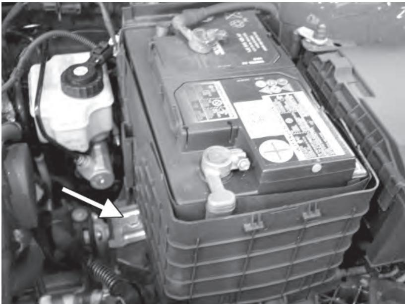
78) Remove the 13mm bolt that holds the battery bracket in place.
