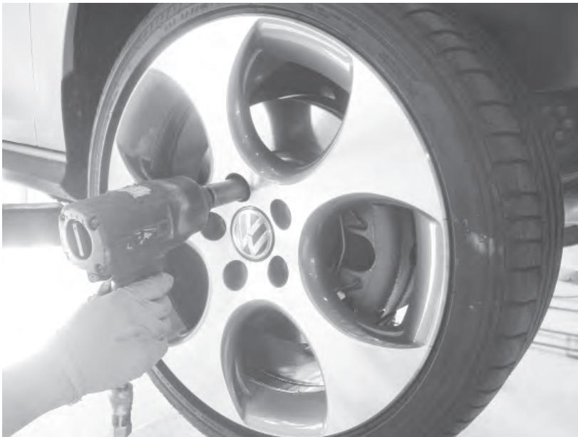
14) Remove the 17mm lug bolts and remove the front passenger wheel and set aside.
