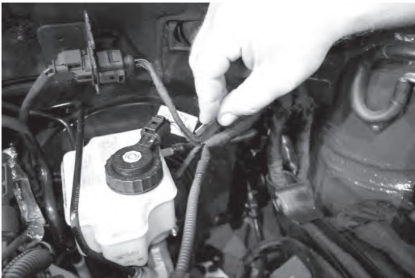
81) Pull the MAF harness tight, and gently cut away the electrical tape where it joins with other harnesses. Be very careful not to cut or slice any wires or wire insulation.
