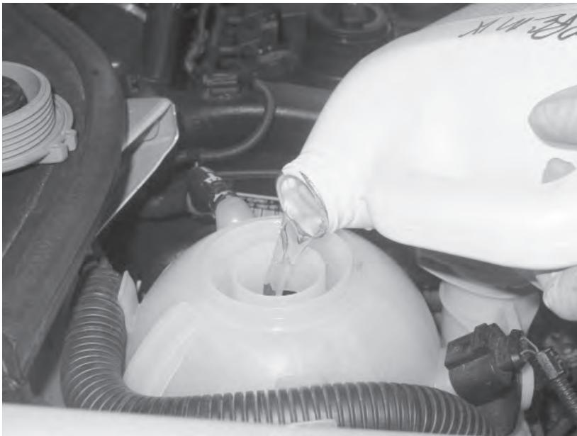
98) Check the engine coolant level and fill if necessary. Reinstall the reservoir cap before the thermostat on the car opens.
