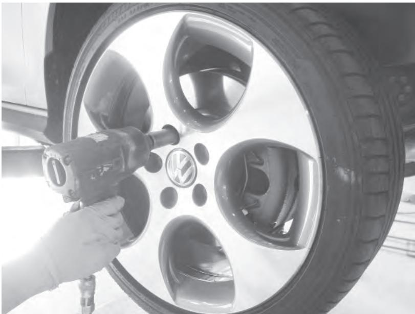
93) Reinstall the front passenger wheel and torque the lug bolts to 89lb-ft.
