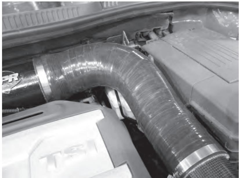
92) Reinstall both the driver and passenger side wheel well liners with the stock T25 screws. Leave the belly pan off for the initial testdrive, so you can check for leaks or reinstall the intercooler hose that blew off that you didn't tighten enough.
