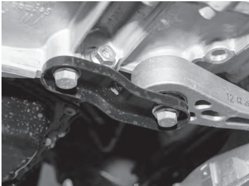
26) Disconnect the transmission dogbone mount from the engine by taking off the two front 16mm bolts.
