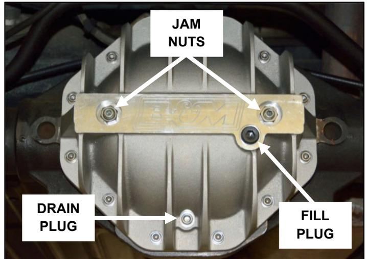
16. Fill the differential with manufacturer-specified gear oil. The bottom of the fill hole is the proper level.
