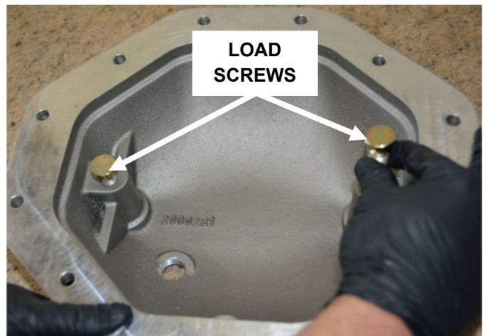
11. Apply gear oil-compatible RTV silicone sealant to the flange of the B&M differential cover. Run the sealant between the screw holes and the inside edge of the flange.
