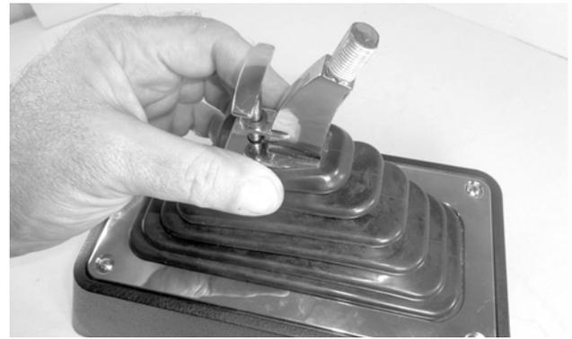
9. Gently work the rubber boot down over the stick and work the boot's lower groove onto the chrome cover. Then work the boot's upper groove onto the stick's lower flange. (The stick has 2 flanges, and the top flange will sit atop the boot.)
