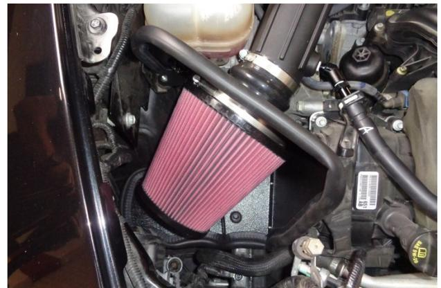
29. Slip screw clamp (2) onto air filter (1), then install the filter on the filter adapter and tighten the clamp.
