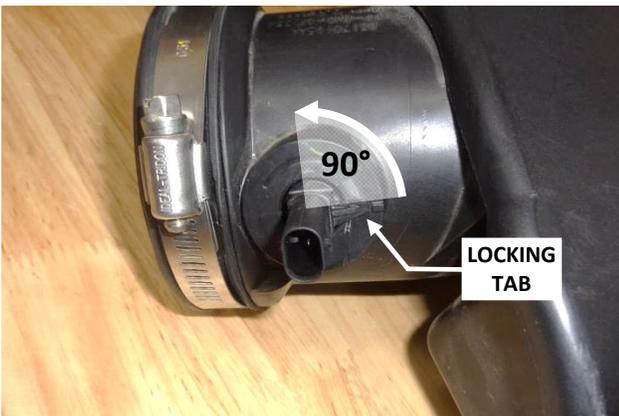
14. To remove the inlet air temperature sensor from the resonator, lift its locking tab, rotate the sensor a quarter-turn counter-clockwise, then pull. Remove the o-ring from the sensor. **CAUTION: The sensor is delicate!** Handle it with care, and store it in a safe location until reinstallation.
