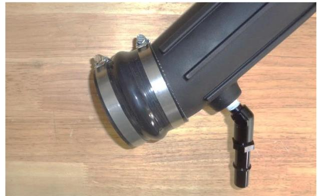
22. Slip the two large screw clamps (9) onto the large coupler (10). Push the coupler onto the intake tube, and snug – do not tighten – only the tube clamp at this time. (Leave the other clamp loose.)
