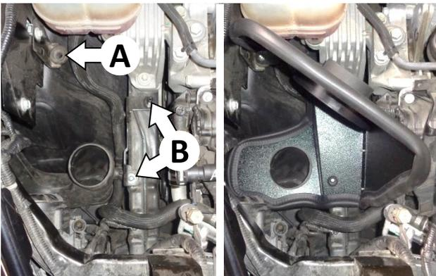
19. Install the heat shield in the vehicle, pushing the barbed pin into the rubber grommet (A), and pushing the rubber grommets over the pins (B). (Moistening the grommets with soapy water will ease insertion of the pins.)
