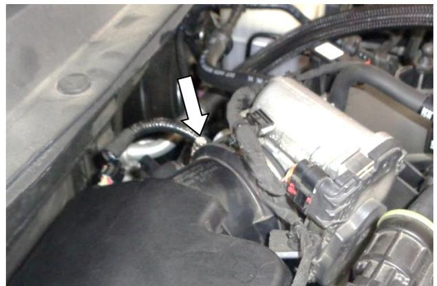
6. Loosen the screw clamp securing the intake duct to the throttle body.
