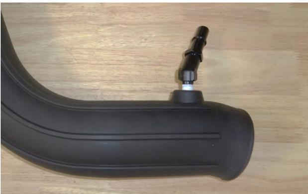
20. Apply 2 wraps of nylon thread tape to the elbow (13) and quick connect fitting (14). Install the quick connect fitting in the elbow, then install the elbow in the intake tube (11).
