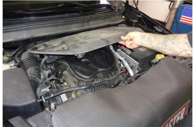
4. Remove the engine cover from the vehicle.
