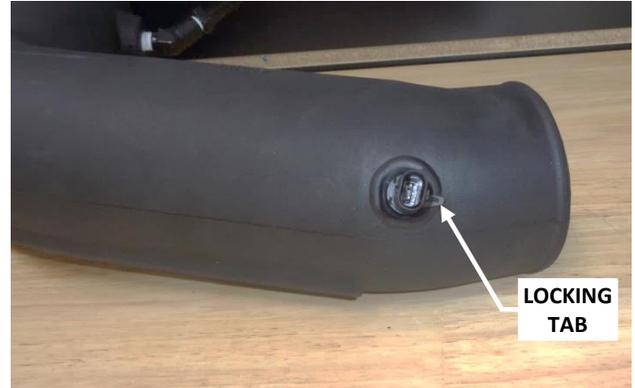
21. Install grommet (12) in intake tube. Carefully push the air temp sensor into the grommet and point the locking tab toward the end of the tube. (Moistening the holes with soapy water will ease insertion of the grommet and sensor.)
