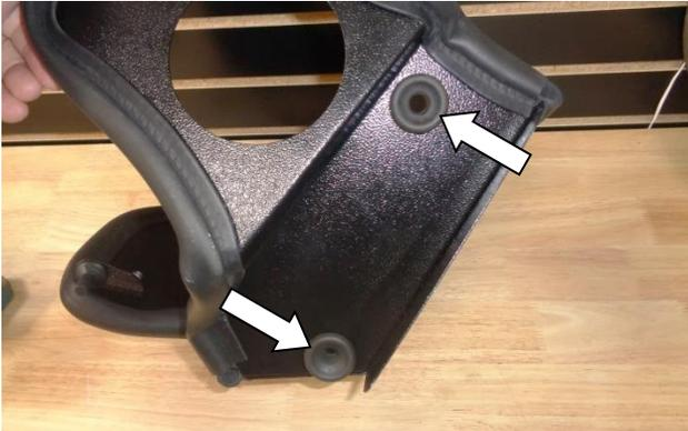
18. Carefully remove the two rubber grommets from the stock airbox, and insert them in the holes on the bottom of the heat shield with the wide openings facing down. (Moistening the holes with soapy water will ease insertion of the grommets.)
