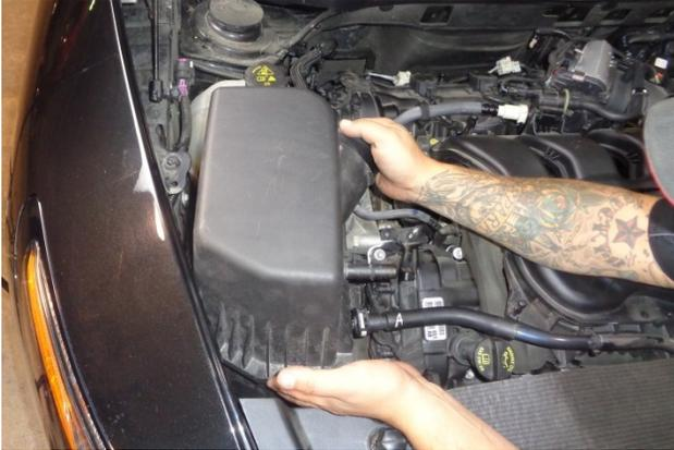
13. Lift the airbox straight up to release its three mount pins from their rubber grommets, and remove it from the vehicle.
