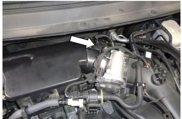
5. Disconnect the electrical plug from the inlet air temperature sensor by squeezing the locking tab, then pulling the plug straight off the sensor.
