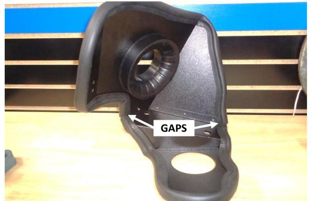
16. Attach the gasket (5) to the heat shield in two pieces, with gaps at the two corners shown. Firmly press the gasket onto the heat shield, gradually working your way around. Use metal-cutting shears to cut the gasket to fit.
