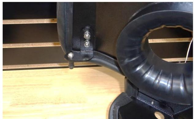
17. Attach bracket (17) to the heat shield using two 1/4-20 screws (19) and flat washers (20) (against the heat shield), and lock washers (21) and nuts (22) (against the bracket). Then attach the barbed pin (18) to the bracket using M6 screw (8), flat washer (7), and lock washer (6).
