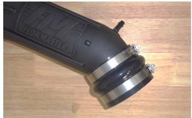
23. Slip the two small screw clamps (15) onto the small coupler (16). Push the coupler onto the intake tube, and snug – do not tighten – only the tube clamp at this time. (Leave the other clamp loose.)
