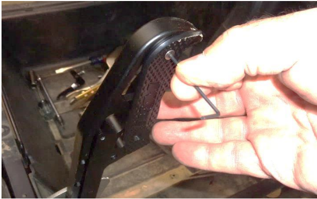
20. Remove both side plates.
