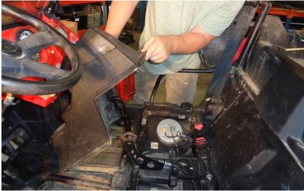
21. Install the center console.
