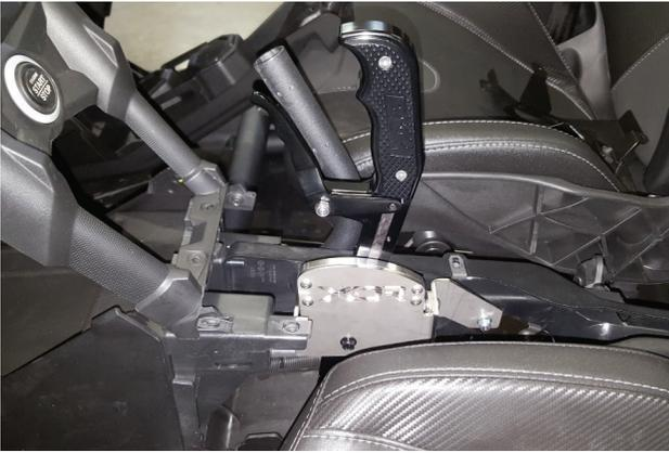
36. Now that shifter components have been assembled, go back and completely tighten fasteners from the previous steps in this order: Steps 33, 34, 35, 32.
